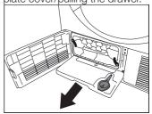
2-Drain the water in the tank
